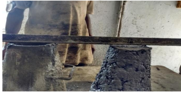
Fig4.1: Slump cone test
