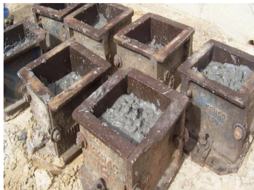
Figure 3.3. Casting of cubes
