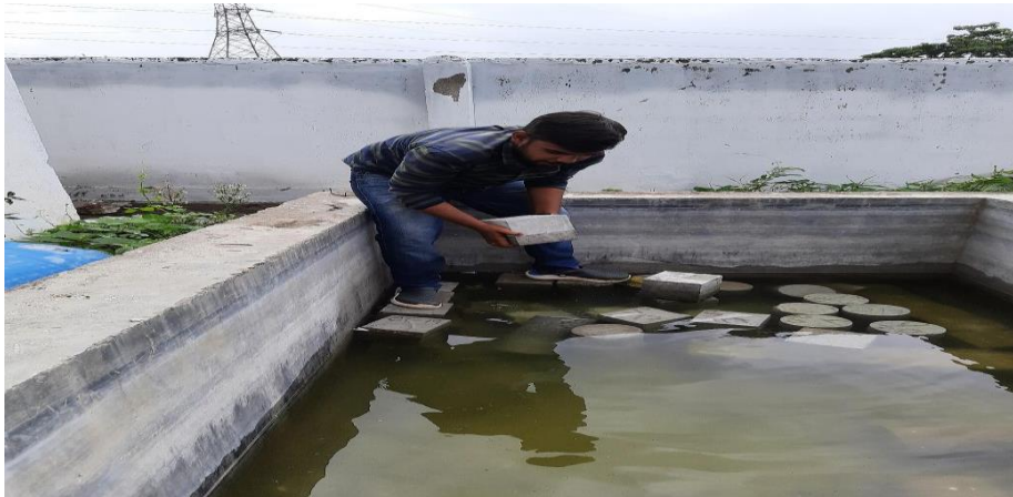
Figure-3.5 Curing of cubes
