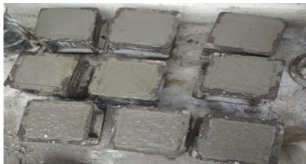
Figure-3.4 Casting of cubes
