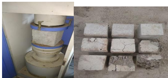
Fig 4.6 compressive testing machine and cubes after test
