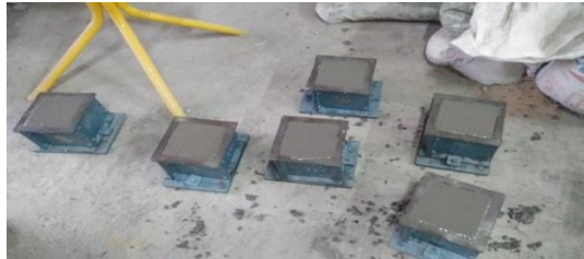
Fig 4.5 casting the cubes
