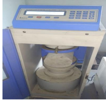
Fig 4.7 Split tensile strength test
