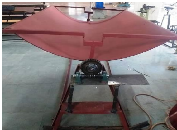
Figure.2. Mild steel fabricated structure of PTC.
