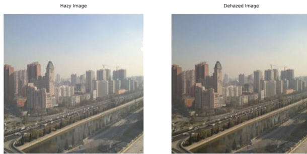
Fig. 6. Hazy Image and Dehazed Image by GAN based Dehazing
