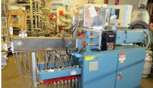
Figure 2. Co-Rotating twin-screw extruder(SB)
