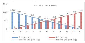
Figure 5.Composition of R1-R2 (polycarbonate resins) blends
