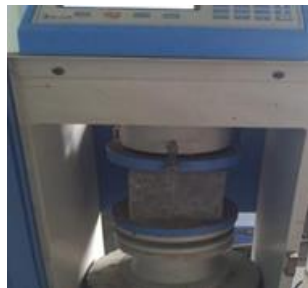
Fig.2.6: Compressive strength testing machine
