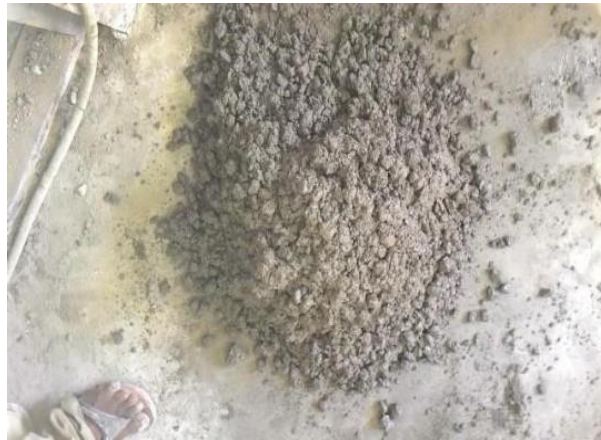
Fig.2.3: Mixing of Recycled aggregate concrete
