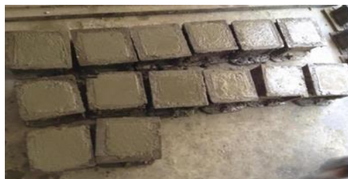
Fig.2.4: Mixing and casting of fresh concrete
