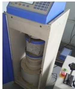
Fig..3.1 Compressive Strength Test of Cubes
