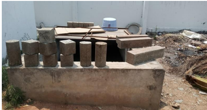
Fig 3.6 Specimens which are kept outside to expose to atmosphere
