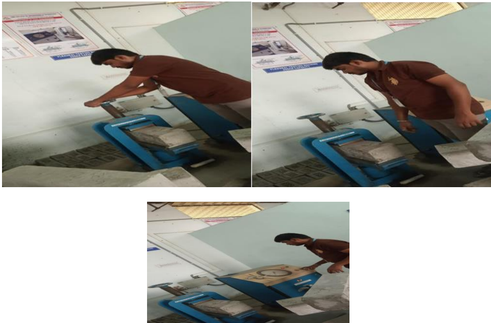
Fig 4.4 Flexural strength test.
