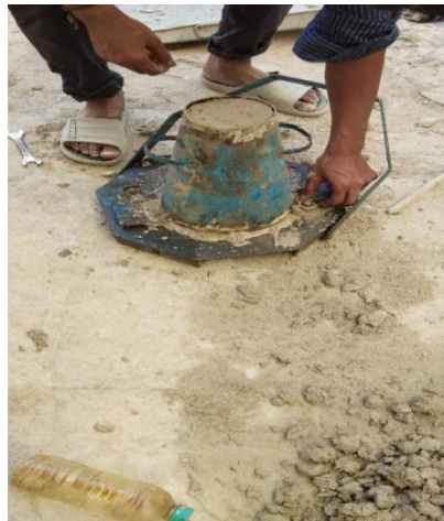
Fig 4.1 Slump cone test
