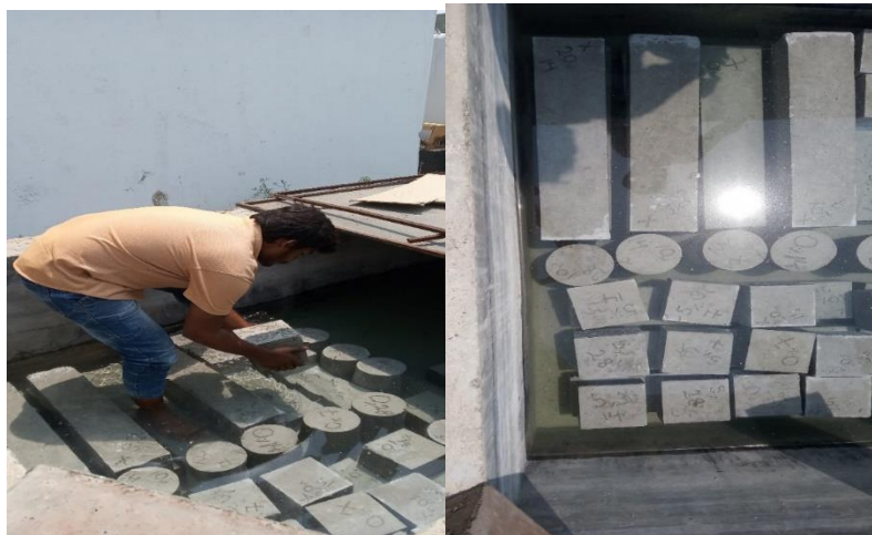
Fig 3.7 Curing of cubes, beams and cylinders
