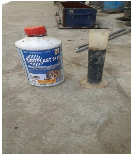
Fig 2.6 Admixture roofplast sp 45
