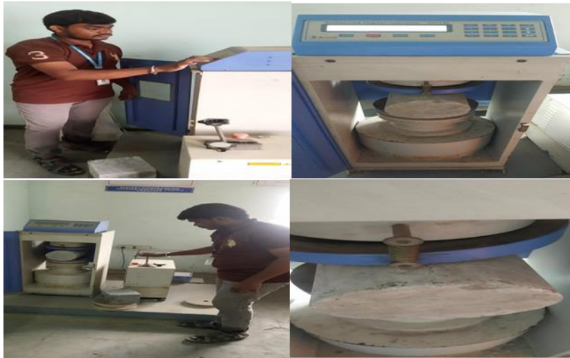
Fig 4.5 split tensile strength test
