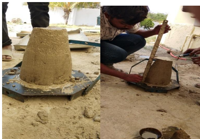
Fig 4.2 Measuring the slump valve
