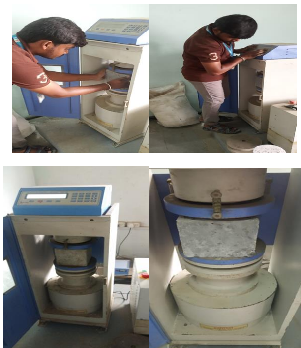
Fig 4.3 Compressive strength test
