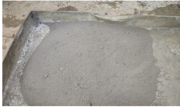
FIG. 2.1. Flyash from Ramagundam Power Station, Telangana
