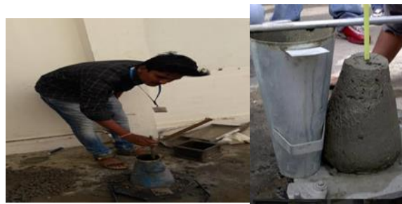
Fig 3.5 workability of concrete
