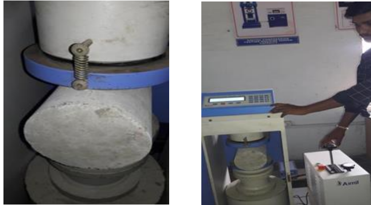
Fig 3.7. split tensile strength of cylinder
