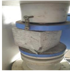
Fig 3.6. compressive strength of cube
