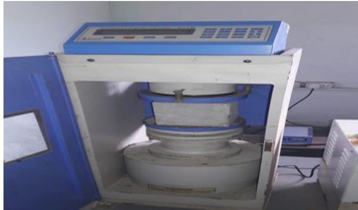
Figure 4.1 compression test of cubes
