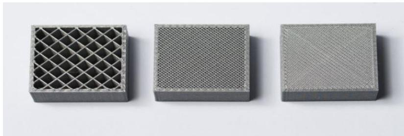
**Fig 3. Various infill density like 50%, 75% and 100%**
