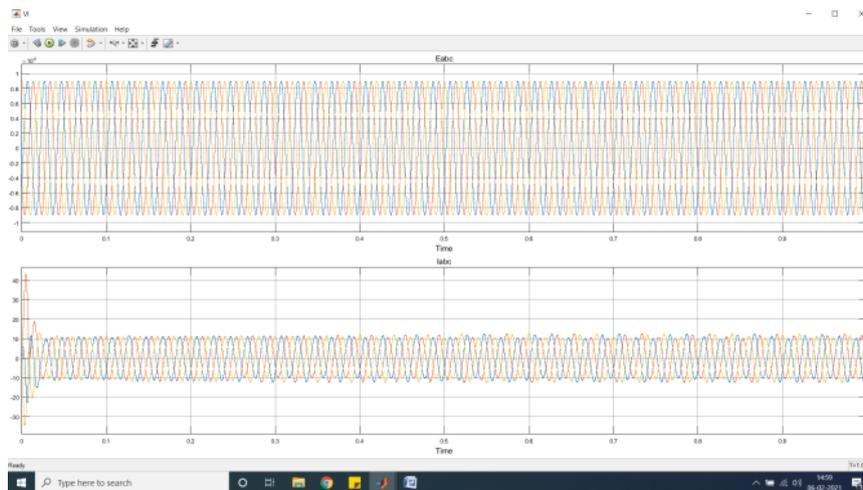
**Fig. 10: Three phase voltages and currents of the inverter with only PVA and WF**
