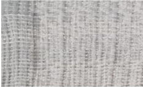
Figure 11, the details of alternately two wefts into single piece of weaving
