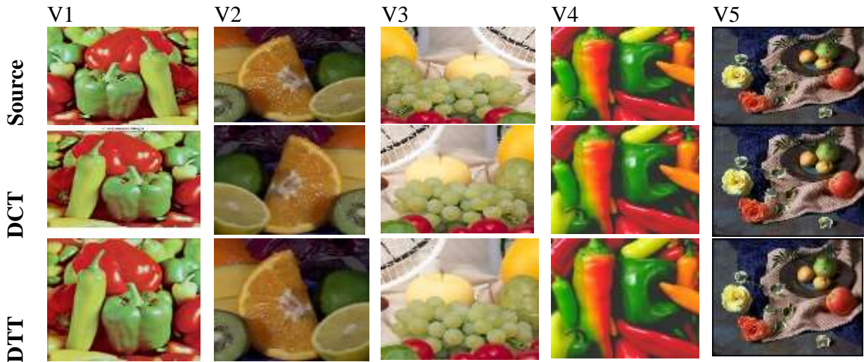
Fig. 5(a) Comparison between DCT and DTT based on compressed Fruits and Vegetables images
