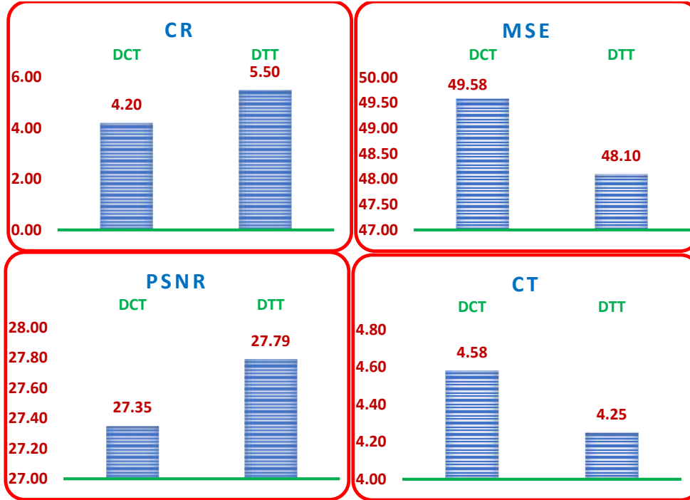
Fig. 5(b) Comparison between DCT and DTT based on CR and MSE for Fruits and Vegetables images
