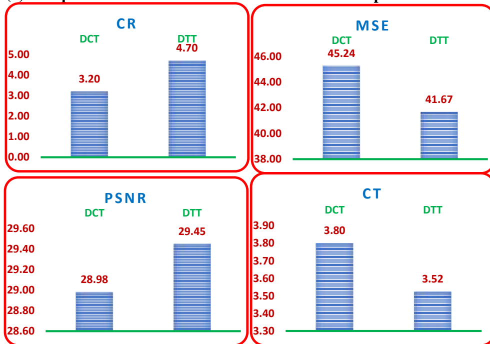
Fig. 4(a) Comparison between DCT and DTT based on compressed Natural images
