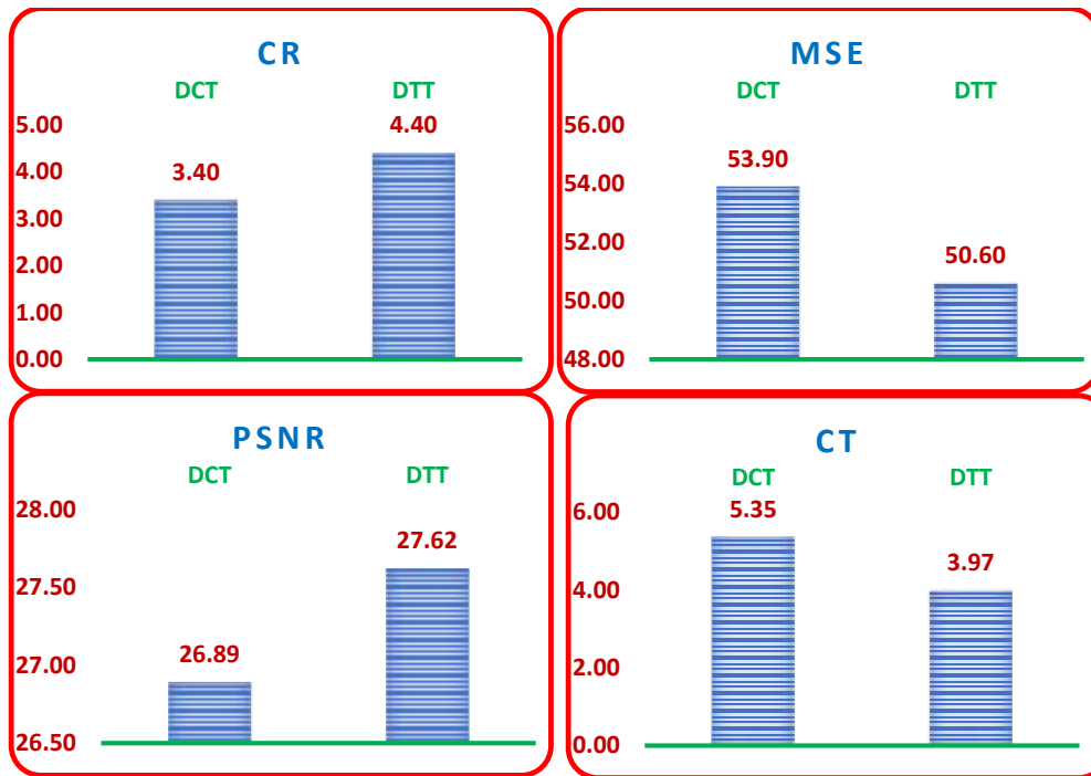
Fig. 1(b) Comparison between DCT and DTT based on CR and MSE for Animals images
