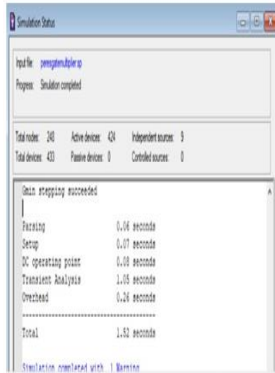
Fig 3: Transistor count output for PFAG multiplier circuit
