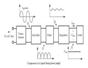
Fig. 8. Components of a typical linear power supply
