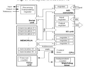
Fig. 2. Block representation of the microcontroller
