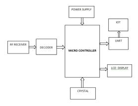
Fig. 4. Block diagram of node 2
