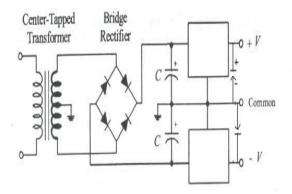
Fig. 9. The basic power supply schematic
