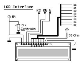
Fig. 5. LCD interface
