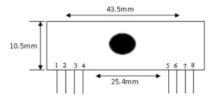
Fig. 7. RWS-434 pin diagram
