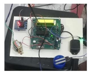
Fig. 12. Flood monitoring electrical circuit node 1
