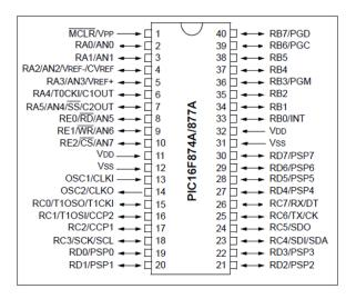
Fig. 1. Pin layout of PIC16f877a
