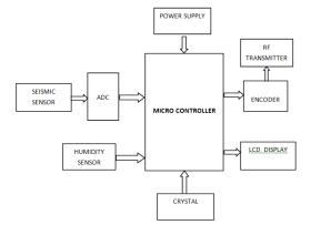
Fig. 3. Block diagram of node 1
