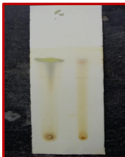
Fig 3.3 TLC with Iodine crystal
