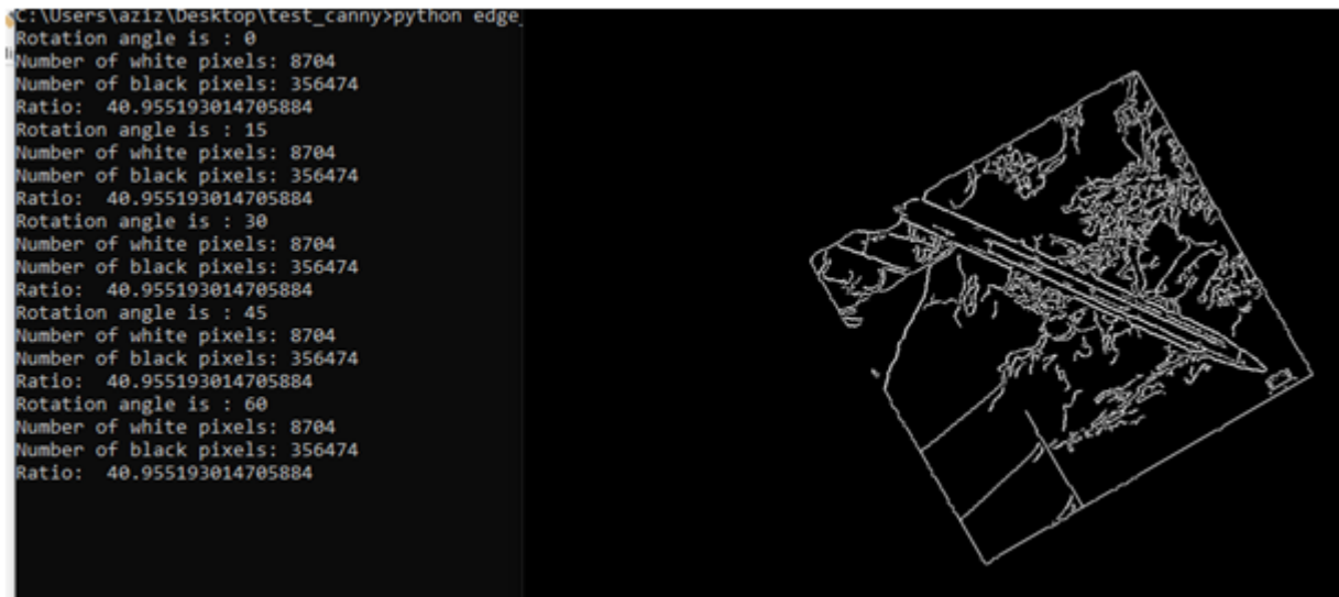
Figure.4 Black-white pixel ratio for a 60 degree inclination.
