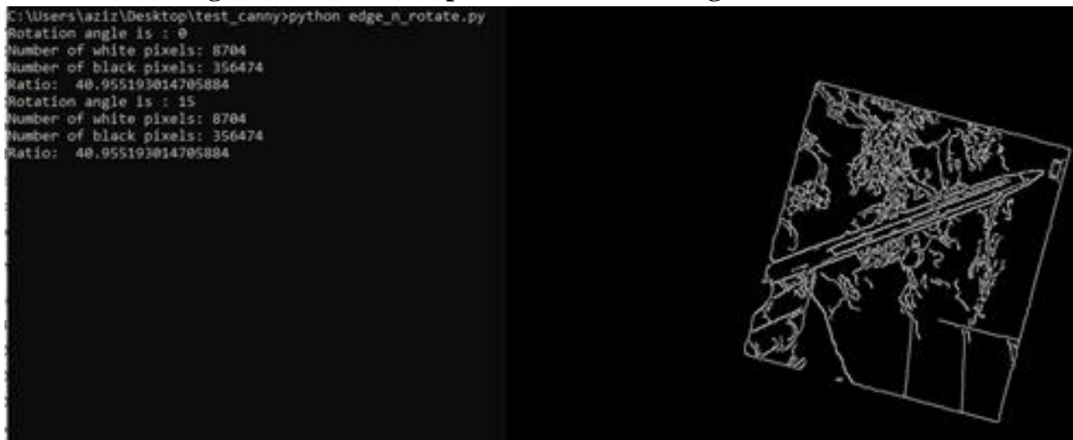
Figure.3 Black-white pixel ratio for a 15 degree inclination.
