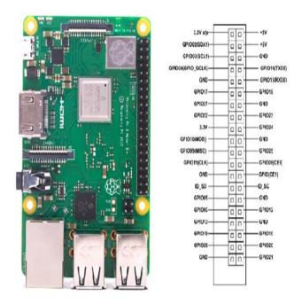
Fig2: Pin diagram of Raspberry PI
