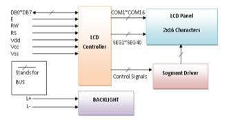
Fig 4 : Block diagram of LCD
