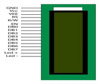
Fig 3: Pin diagram of 6 X 2 LCD
