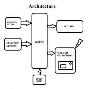
The block diagram has two parts,
