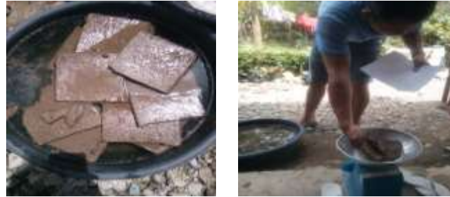
Figure III. Material preparation for swelling test
