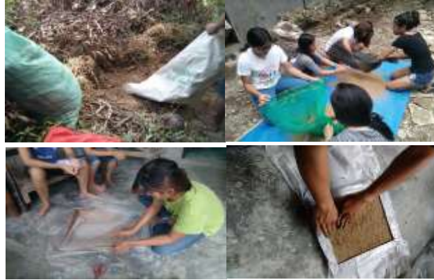
Figure I: Sieving, mixing and molding of Tiger Grass pollen with arrowroot starch as binder
