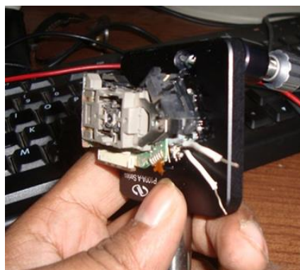
Figure 5. DVD optical pickup's laser diode with wires connected
