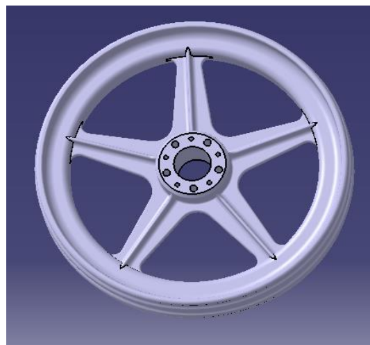
Figure 1. Alloy wheel Design CATIA v5 Software
