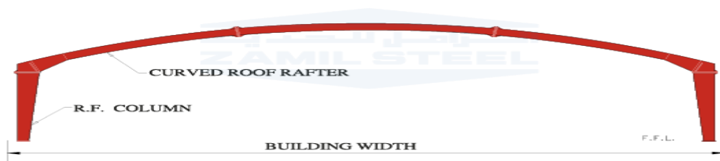
Fig7 :arched clear span
