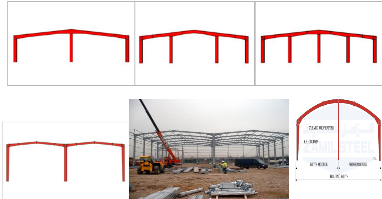
Fig 8 :multi span buildings
