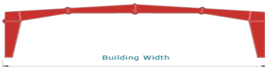
Fig 6 :clear span framing system
