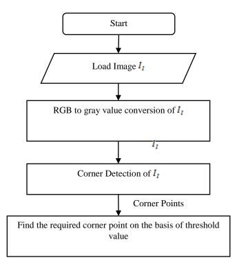
Figure 4: Flow diagram of Harris Corner detection
