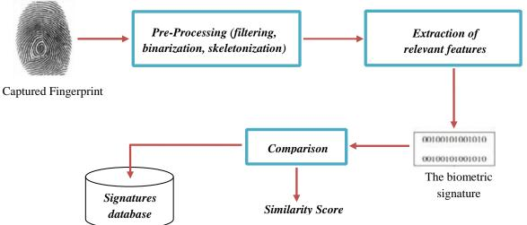
Figure 1: Design of a biometric system based on fingerprints
