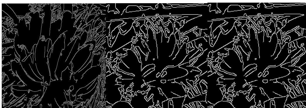
Fig. 5. Images after applying Canny Edge Detection
