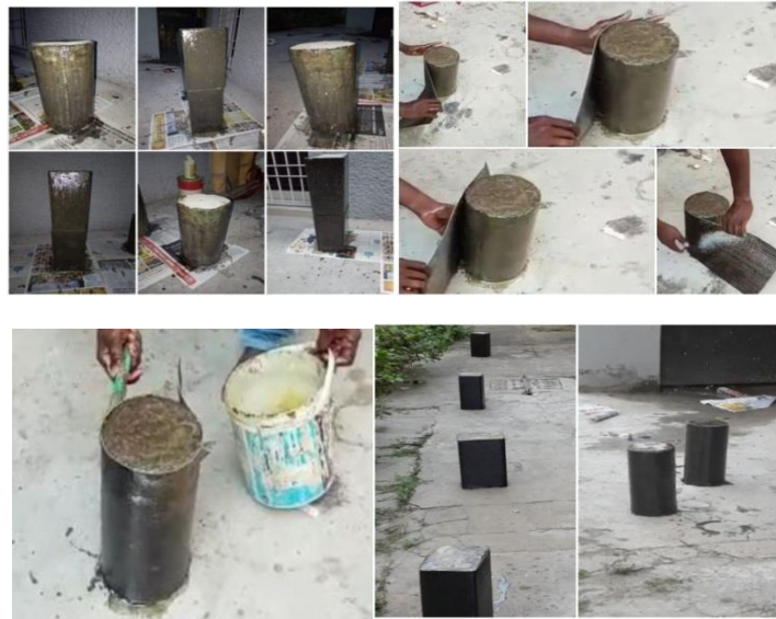
Figure. 3 Process of the CFRP Wrapping
