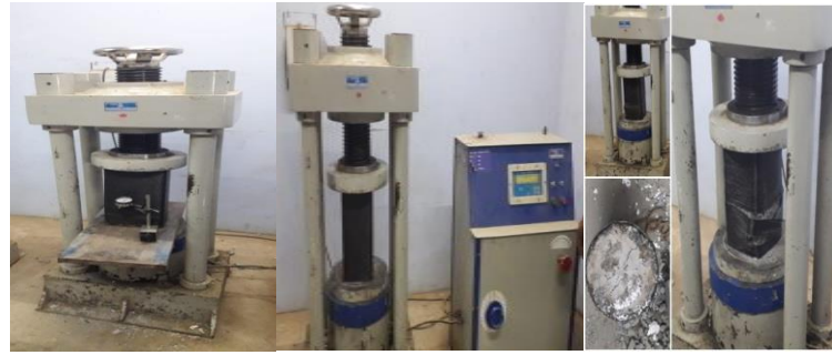
Figure.5 Testing of the Circular Square and Rectangular CFRP wrapped Specimens
