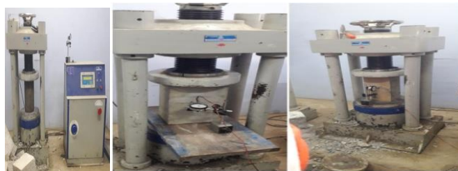
Figure. 4. Testing of the Circular Square and Rectangular conventional Specimens
