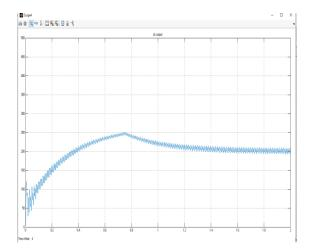
The below waveform shows the efficiency of an dc load with input voltage obtained from bridgeless SEPIC pfc rectifier.
