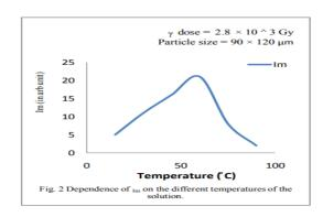
2. Fig.2 shows that the I<sub>m</sub> (maximum intensity) is optimum for the particular temperature of the solution.
