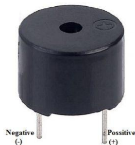
Figure 5: Buzzer pin configuration.
