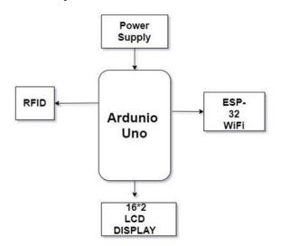
Fig.3 Block Diagram of System
