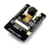
Fig 2:ESP32-CAM with ESP32 chip
