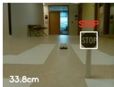
Fig:7 Measure stop Signal within Distance
