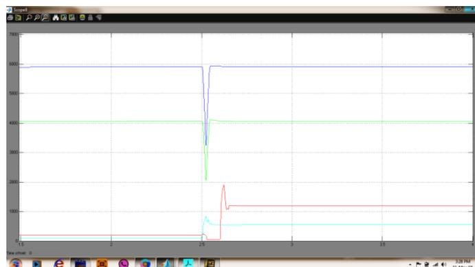
Fig:10. Active Power variation during a 50% primary voltage sag.
