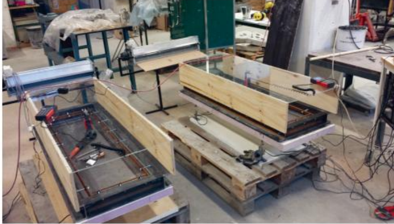
Figure Two rectangular mould test setups with fans and wind tunnels, placed on four load-cells
