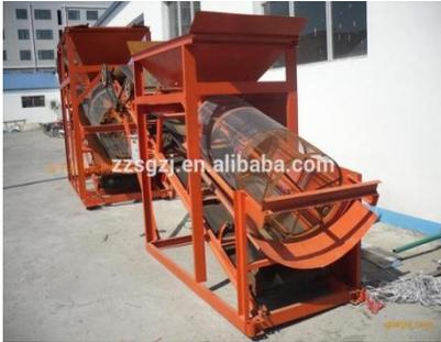
Fig: 1 Hopper with sieve drum
