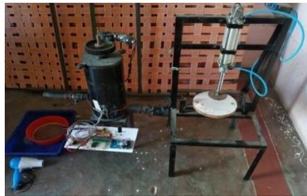
Fig: 2 Assembled figure of paper recycling machine
