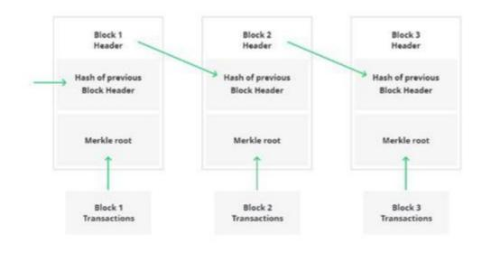
Figure 1: Basic Block chain Structure.
