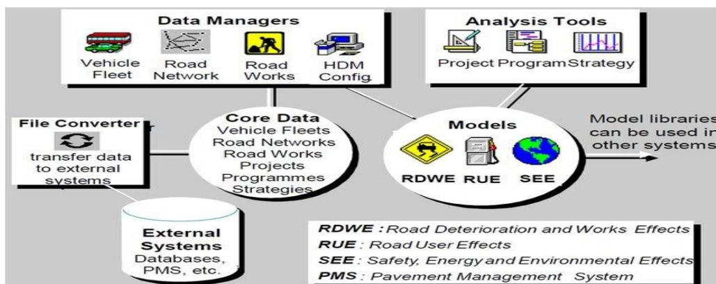
Fig 1: HDM-4 software System Architecture
