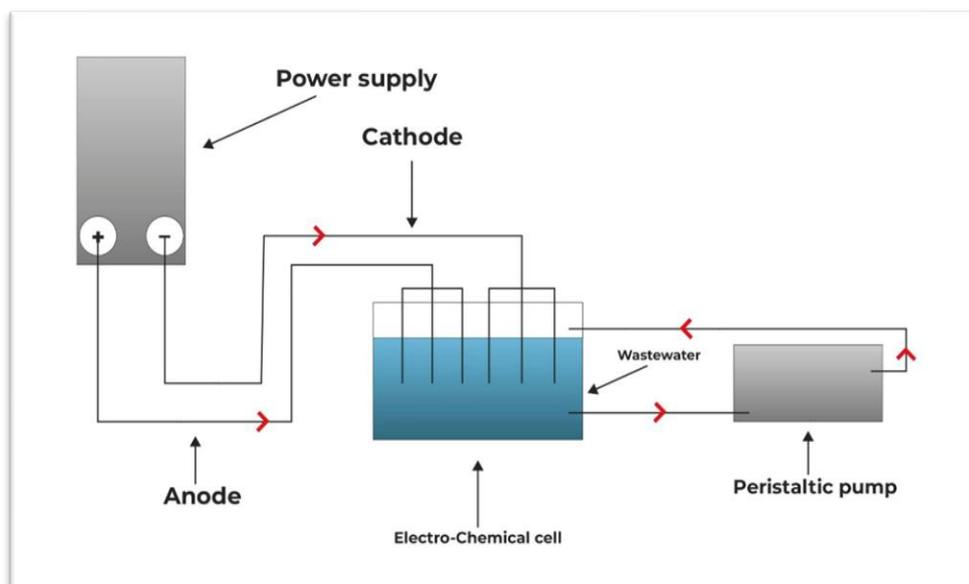
**Fig 2.** Schematic diagram of the EC cell
