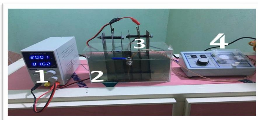
**Fig 1.** A photograph of the EC cell 1. Power supply 2. EC cell. 3.The electrodes (Aluminium and Iron). 4. Pump
