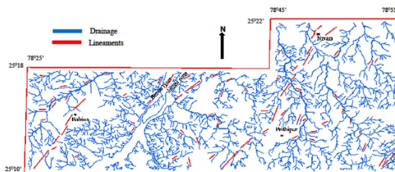
Fig. 4.. Relationship between drainage pattern and major lineaments extracted from various toposheets and IRS- LISS III images in the study area
