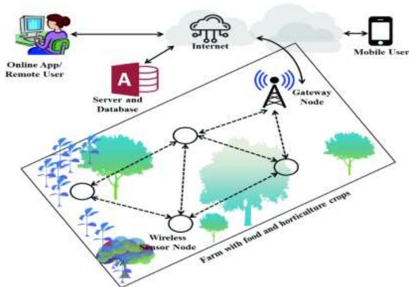
Figure 2. Deploying Wireless Sensor Networks and IoT for Precision Agriculture
