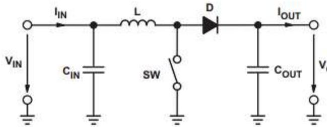
**FIG.5. BASIC CIRCUIT OF BOOST CONVERTER**
