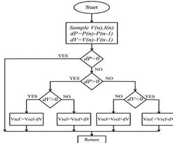
**FIG.3. FLOWCHART OF PERTURB AND OBSERVE METHOD**
