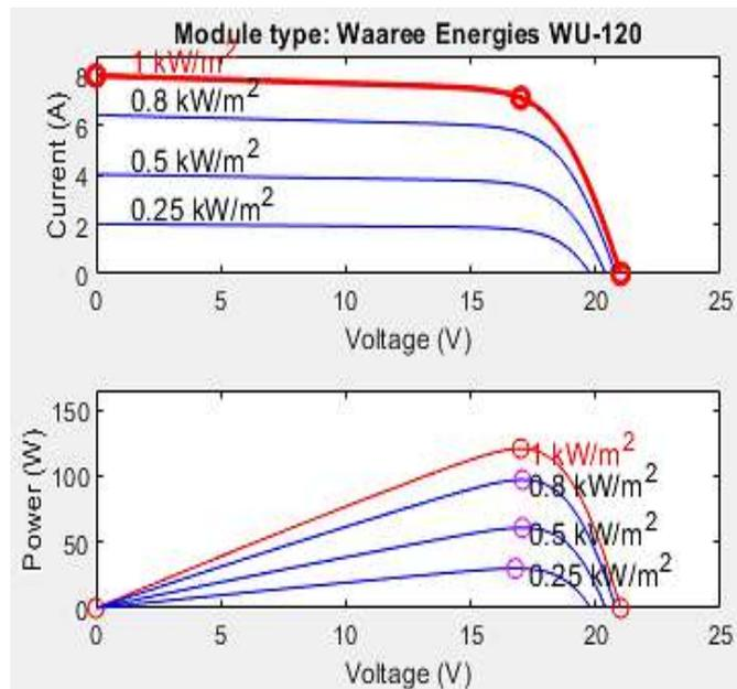
**FIG.2. (a) I-V AND (b) P-V FAMILY CURVES FOR DIFFERENT IRRADIATIONS**
