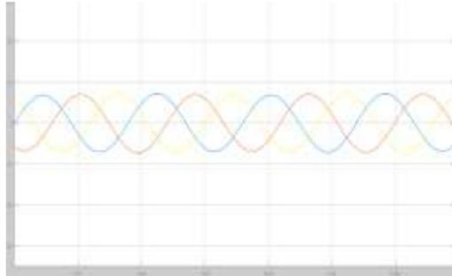
**FIG.15. THREE PHASE INVERTER OUTPUT LINE CURRENTS WAVEFORM**
