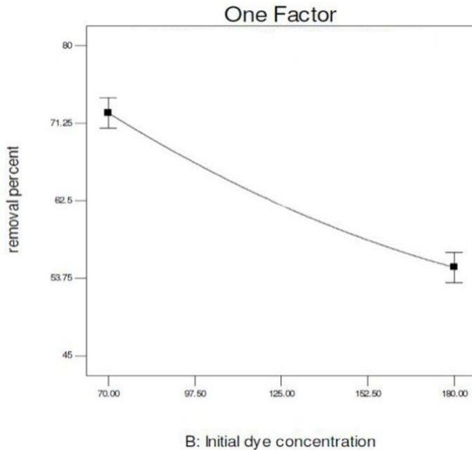
Fig. 5. The effect of initial dye concentration on the dye removal efficiency (retention time = 5 hours)
