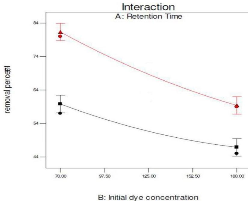
**Fig. 6.** The interaction of retention time and initial dye concentration on the dye removal efficiency (retention time = 3 and 7 hours)
