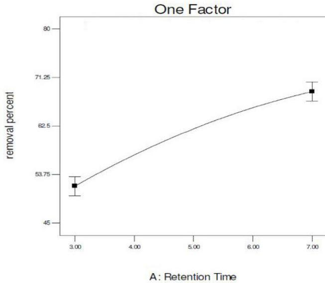
Fig. 4. The effect of retention time on the efficiency of dye removal (input dye concentration = 25 mg/l)
