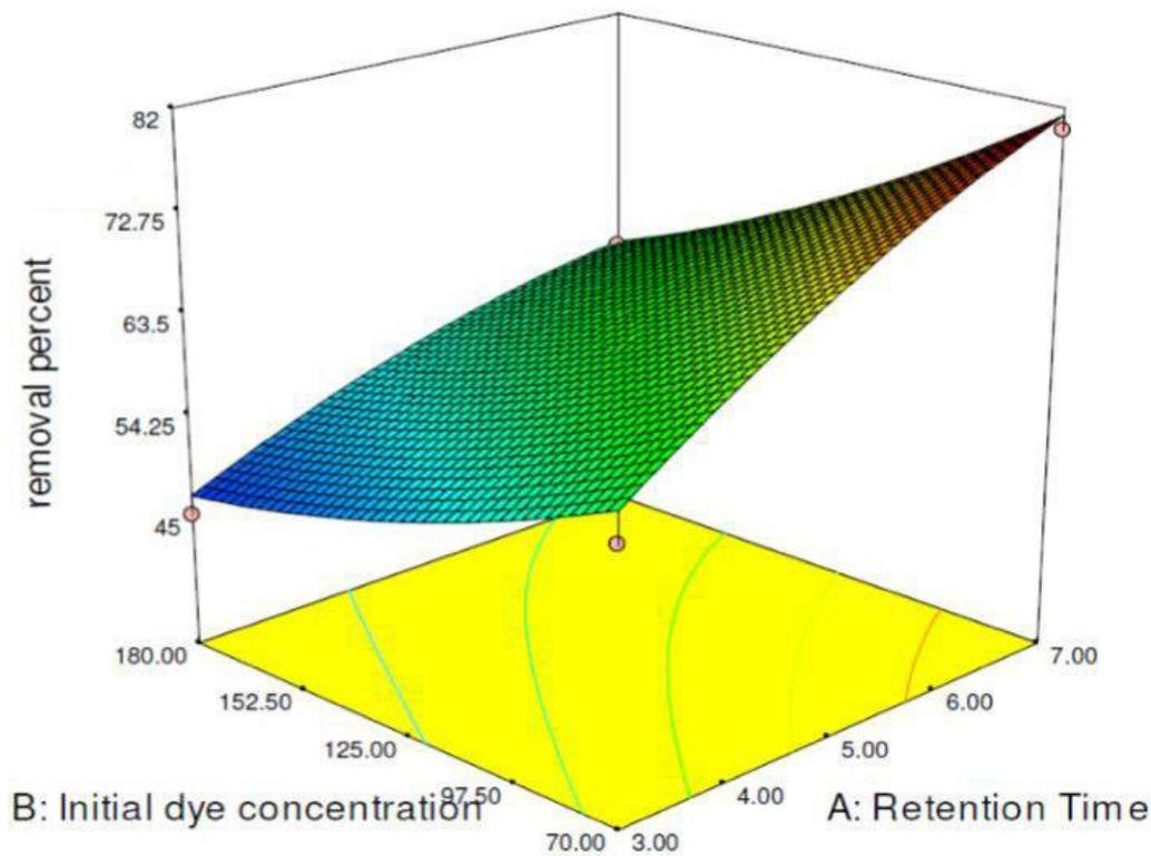
Fig. 3. The effect of retention time and initial dye concentration on the efficiency of dye removal
