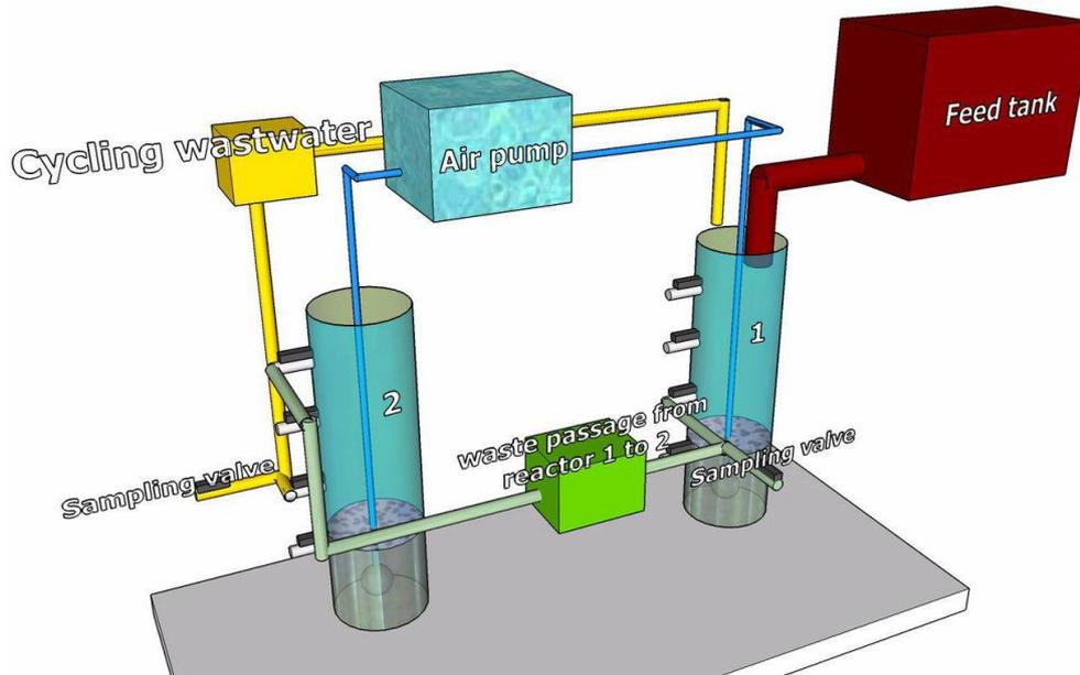
Fig. 2. The three-dimensional schematic view of FB/FFMBBR bioreactor
