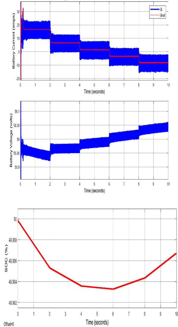
**Figure 10. Voltage, Current and State of Charge of a single Battery**
