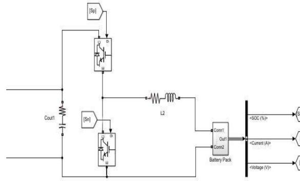
**Figure 6. Charging and discharging circuit**
