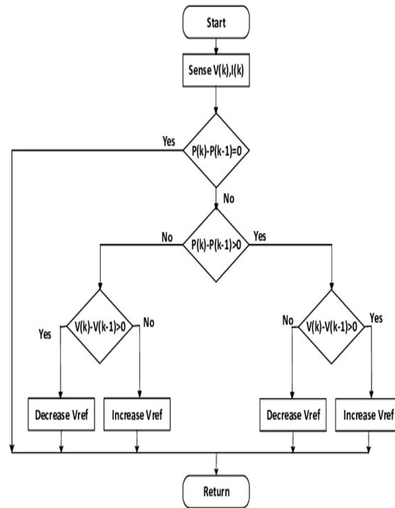
**Figure 5. Step by step algorithm of Perturb and Observe method**
