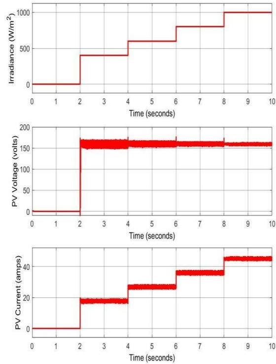
The output parameters of Boost converter and the duty cycle ration generated through Perturb and observe
