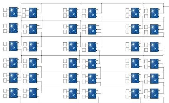
Maximum Power From Tct Configuration Of Pv Array Using P&O Algorithm.
