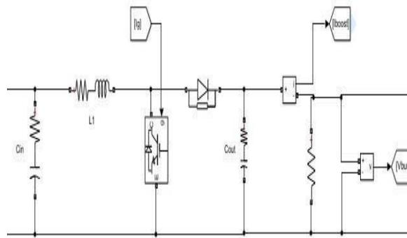
**Figure 4. Boost converter Simulink model**
