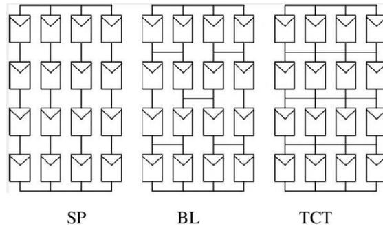
**Figure 1. Different Configurations of PV array**
