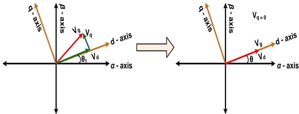
**Fig. 1 Phasor representation of grid voltage on two coordinate axis**
