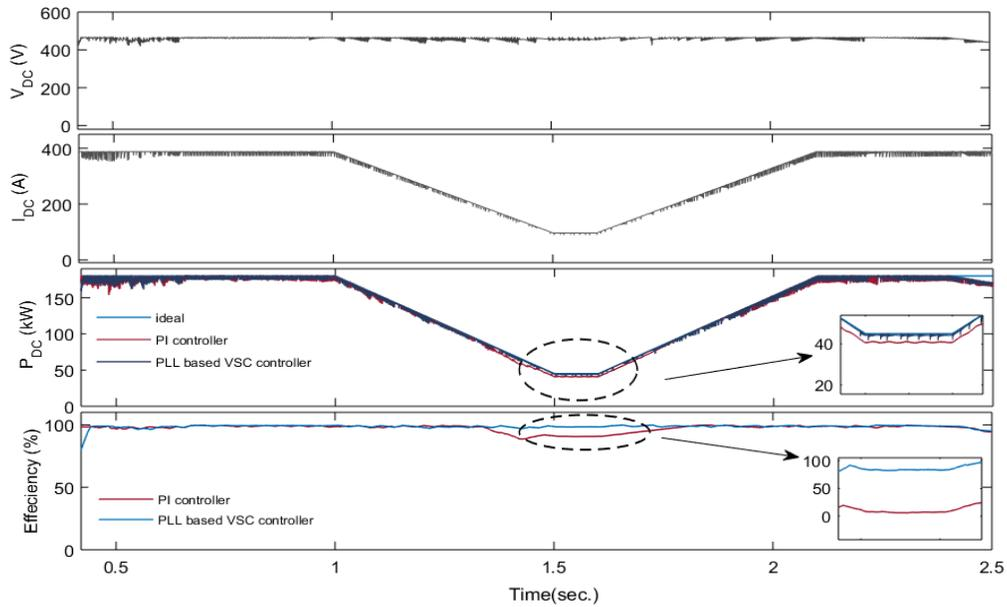
**Fig. 4 DC-link voltage, current, and power under the proposed controller**
