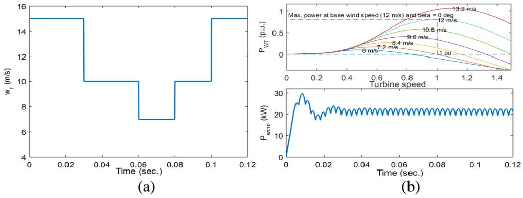
**Fig. 3 Wind speed and wind turbine power characteristic**
