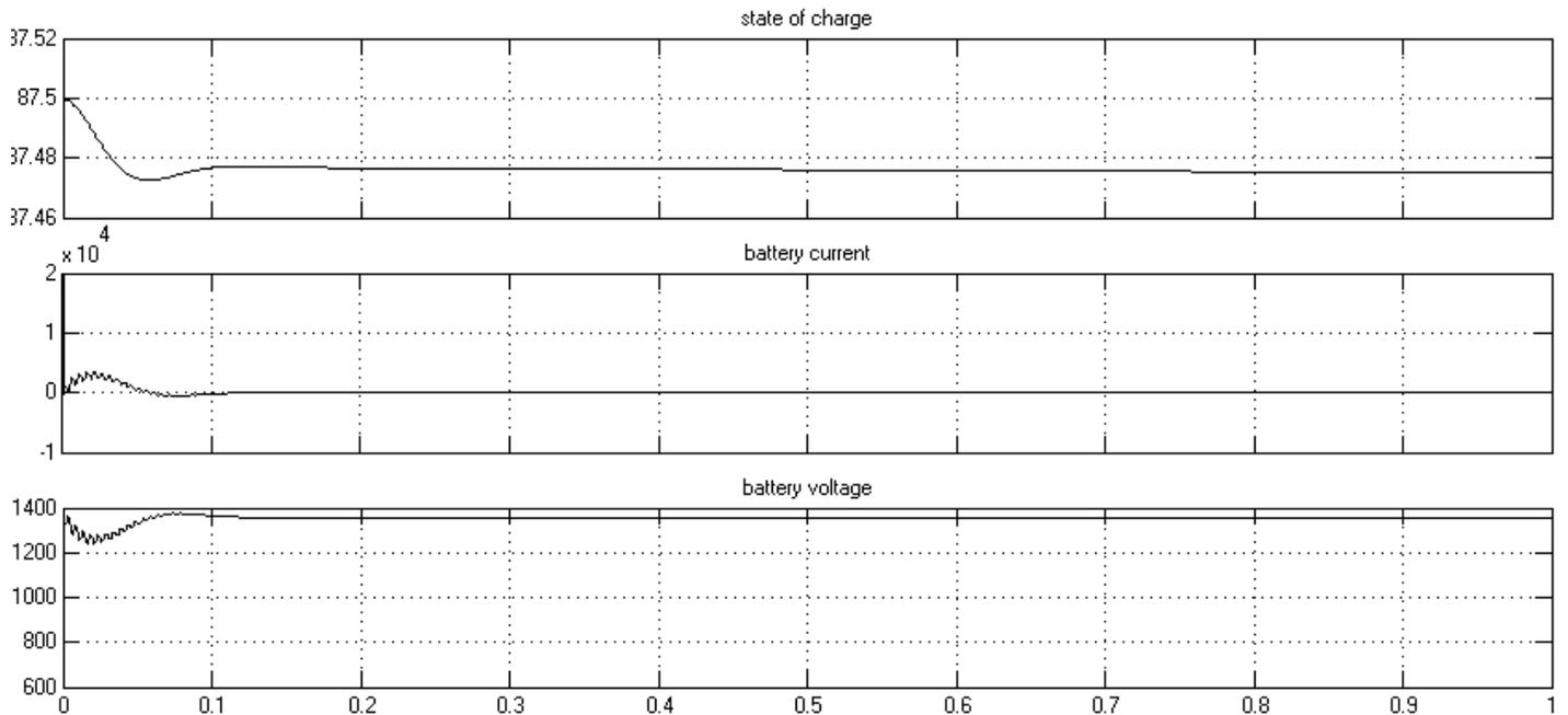
(b) Battery waveforms
