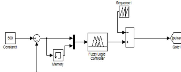
Fig. 4 DC-DC converters using fuzzy logic controllers
