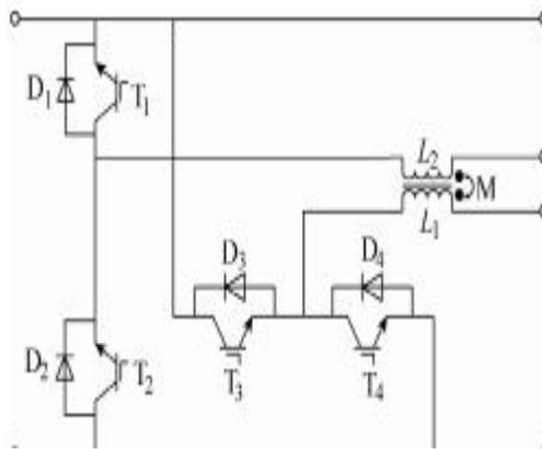
Fig. 2 DC/DC converter topology of the magnetic components
