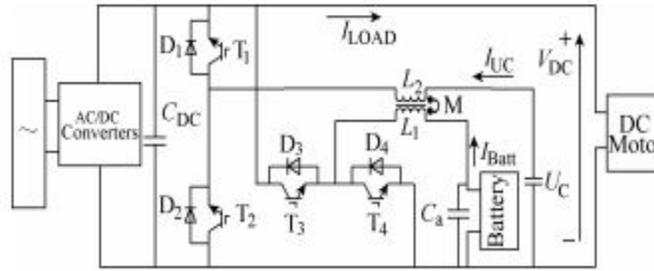
Fig. 1 a hybrid energy storage system's topology
