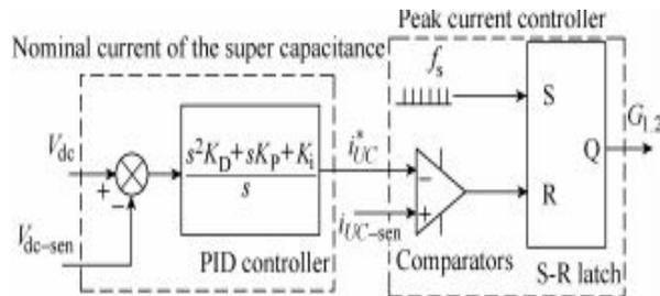
Fig.3 A super-capacitor voltage and current controller's block diagram
